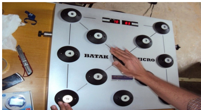
Figure (2) Illuminating Lamps device to measure the speed of the motor response
